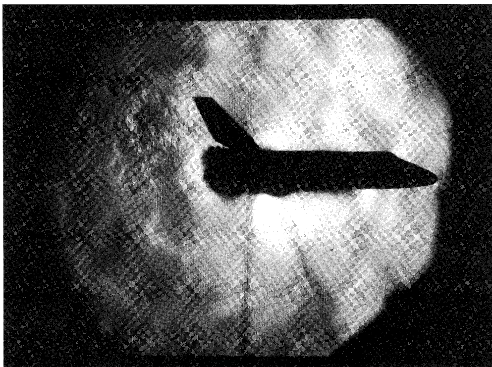
Fig. 6 Modified Space Shuttle model in the 0.3 m TCT; vertical grid, T_t = 120 K, p_t = 5.78 ata, M = 0.5 , R_L = 32.0 \times 10^6 .
