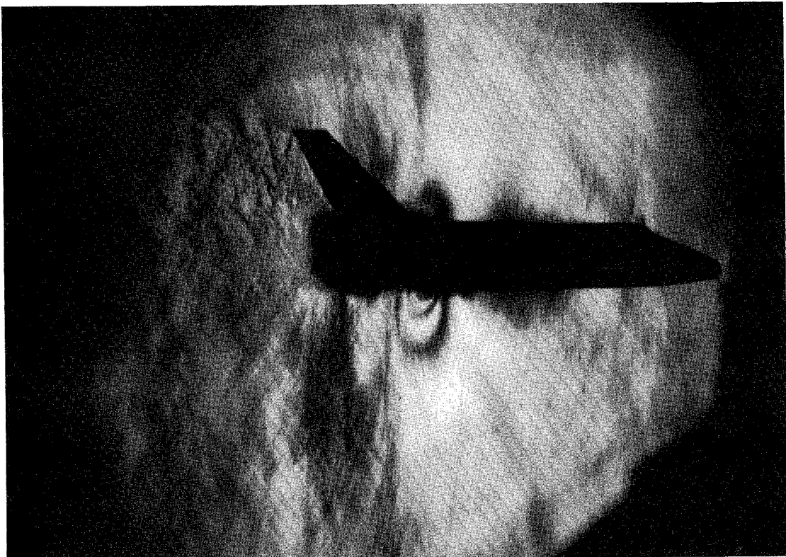
Fig. 8 Modified Space Shuttle model in the 0.3 m TCT; vertical grid, T_t = 120 K, p_t = 5.78 ata, M = 0.85 , R_L = 44.3 \times 10^6 .
