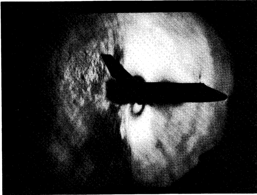
Fig. 7 Modified Space Shuttle model in the 0.3 m TCT; vertical grid, T_t = 120 K, p_t = 2.04 ata, M = 0.85 , R_L = 15.6 \times 10^6 .
